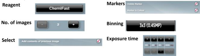
To set up S.A.C select the exposure time for the first and last image then select the total number of images you wish to capture, the level of binning and whether you wish to capture a marker.
